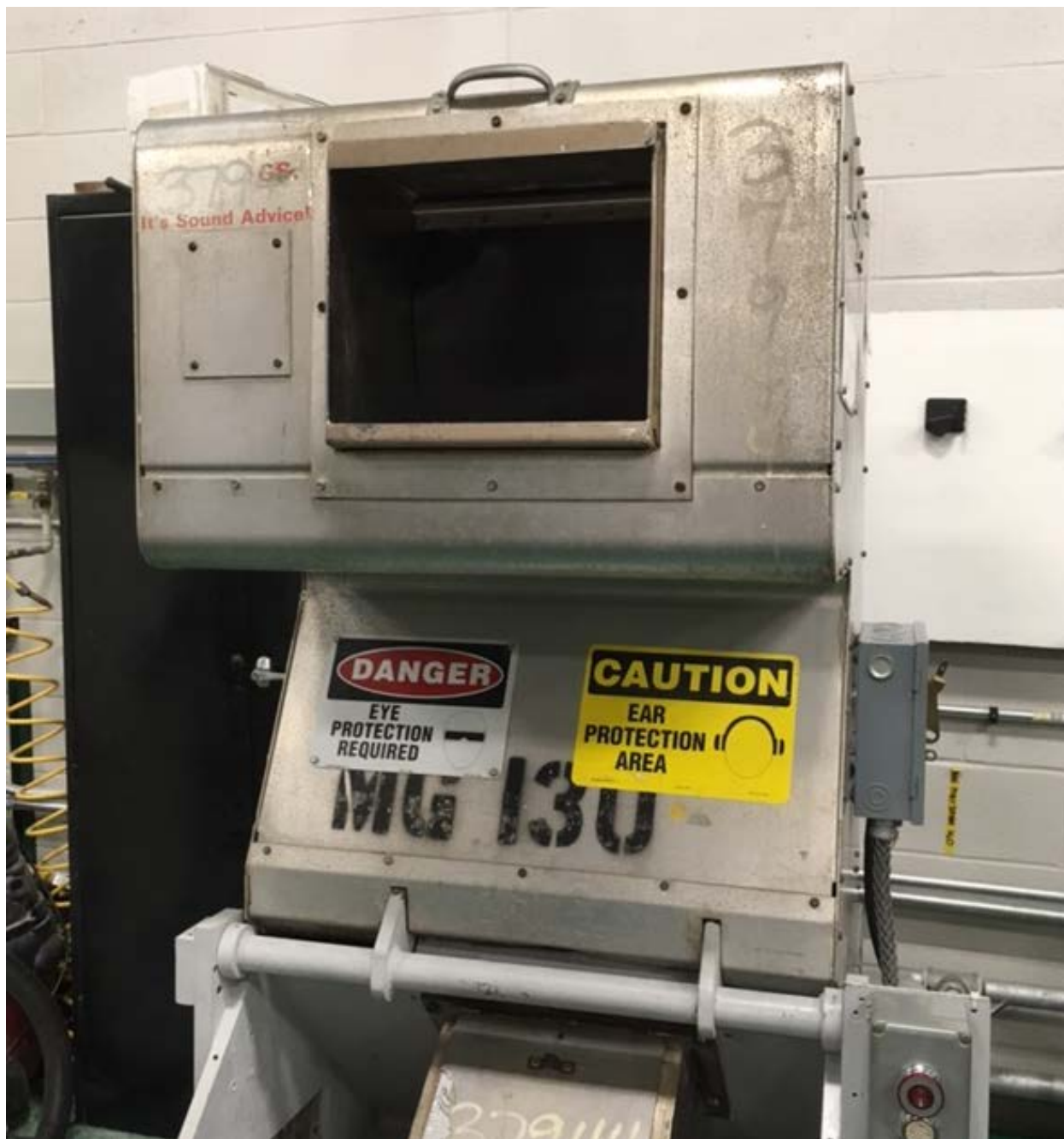
Grinder used in this study using a 3/8" screen
