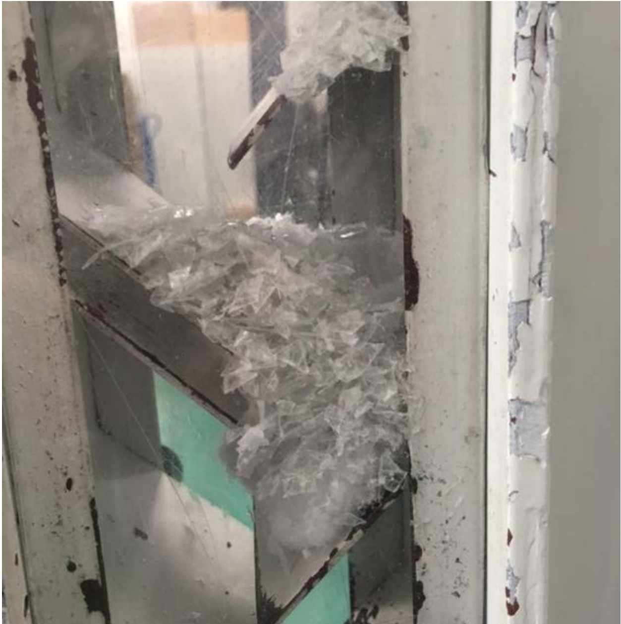
Fibrous material and bottle flake trapped on baffles in the elutriator
