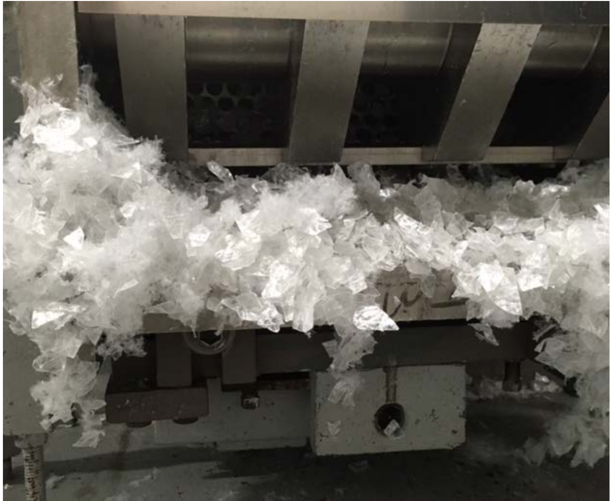
Ground fibrous material with bottle flake built up in the grinder screen
